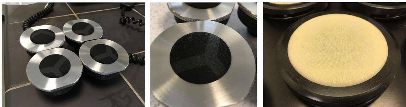
Figure 3.2 Image showing graphene-enhanced fabric before test (left), wear to graphene-enhanced fabric (middle) and abradant material (right).
