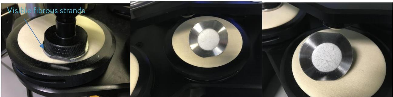
Figure 3.1 Image showing visible fibrous strands (left), wear to baseline fabric (middle) and abradant material (right).
