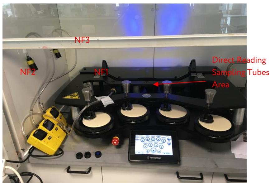
Figure 2.2 Image of Martindale instrument with static sampling and real-time sampling positions outlined
