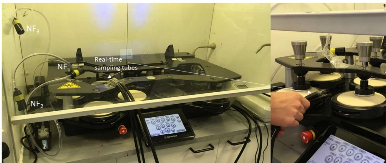
Figure 2.2 Image of Martindale instrument with static sampling and real-time sampling positions outlined
