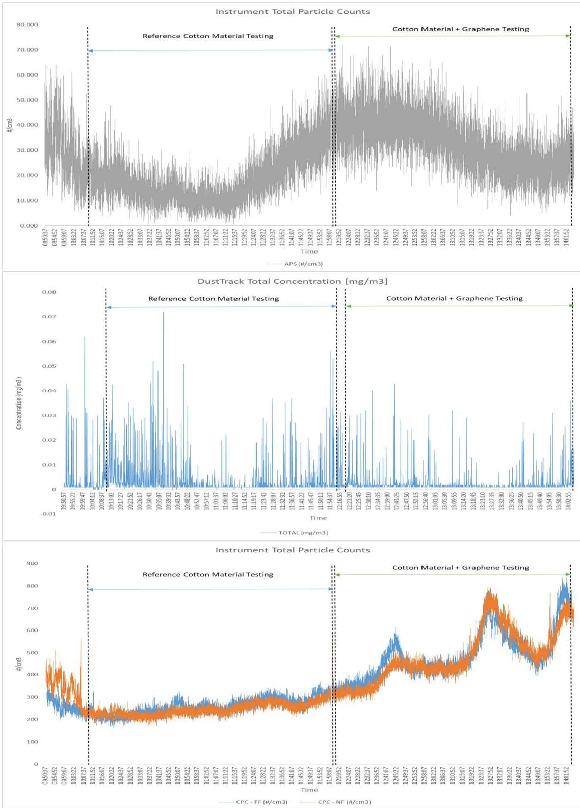
Figure 3.3 Top – APS; Middle – DustTrak particle concentration-time series; Bottom CPC, Abrasion testing. Instrument detection limits outlined in Section 0.
