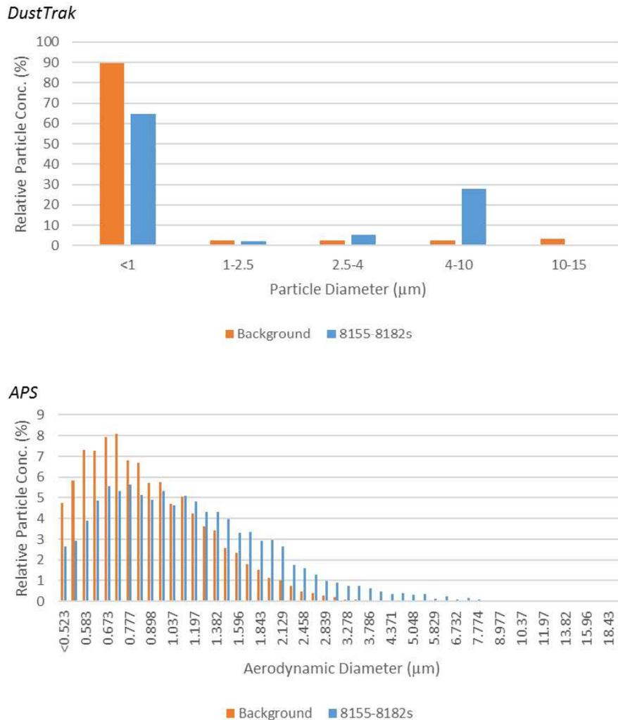
Figure 3.4. DustTrak and APS particle size distribution (PSD) graphs of the peak observed at the start of abrasion testing of graphene-enhanced textile (Figure 2.3, 8155 and 8182 s). DustTrak, size range <1 – 15 µm. APS, size range 500 nm - 1 µm.
