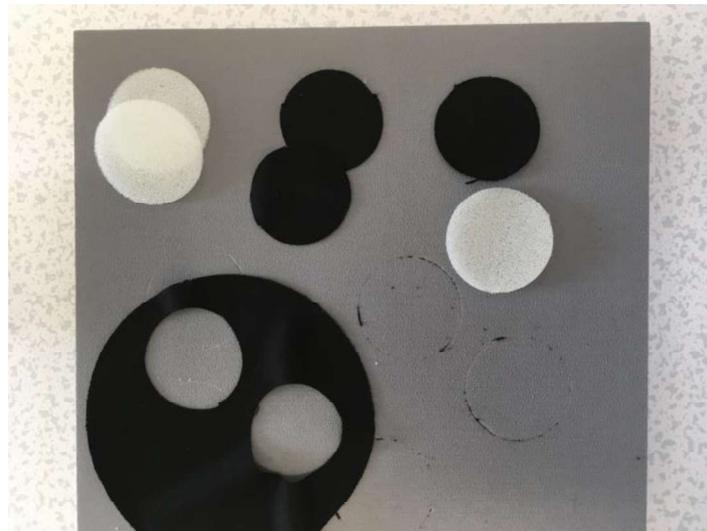
Figure 2.1 Textile samples and polyetherurethane foam inserts cut to correct size
