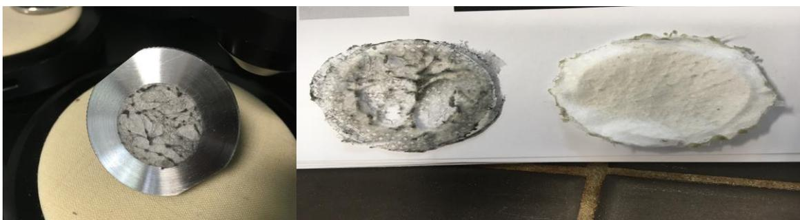
Figure 3.2 Image showing wear to graphene-enhanced fabric post-test (left) and post testing abradant materials (right).
