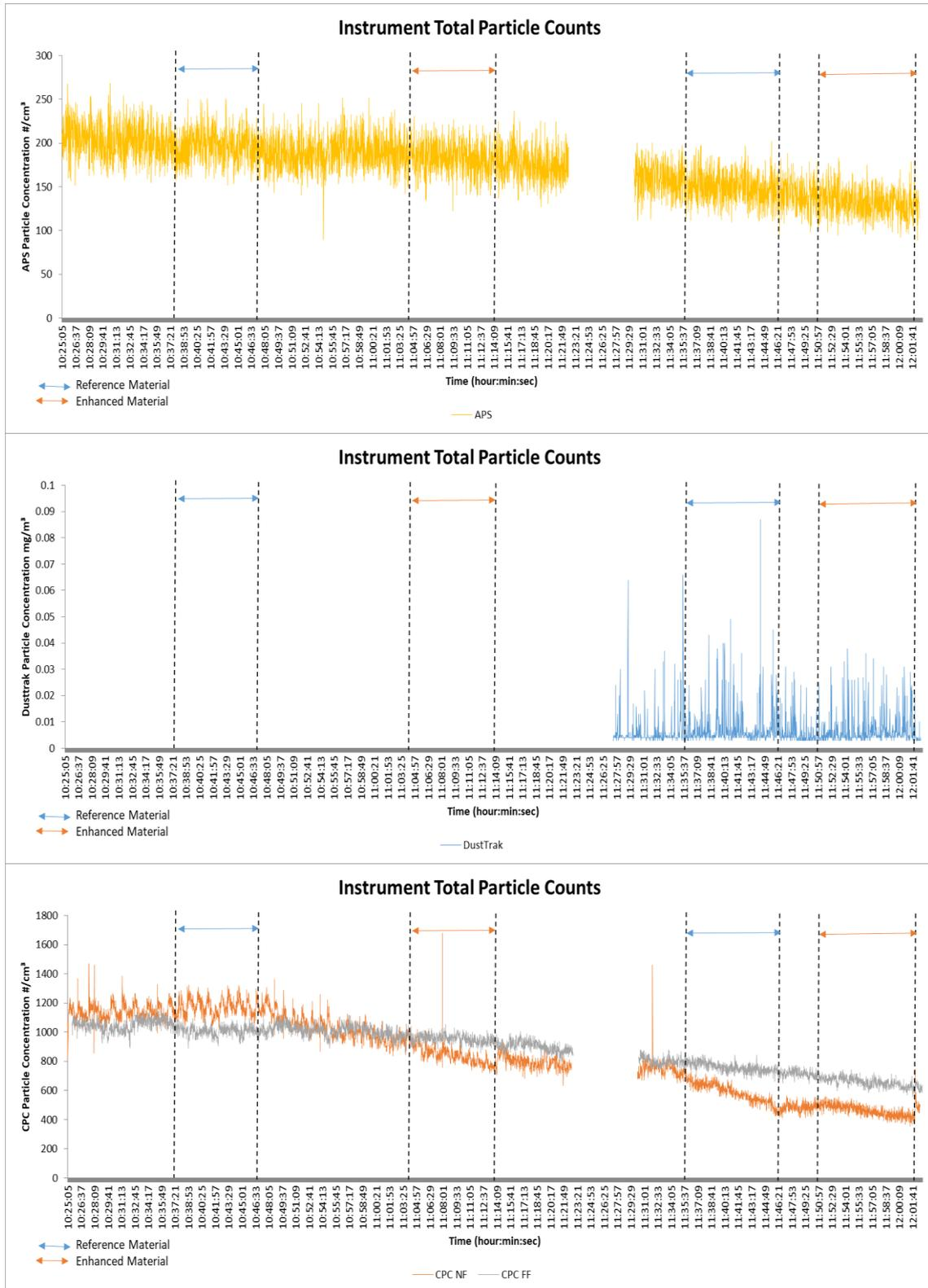
Figure 3.3 Top – APS; Middle – DustTrak particle concentration-time series (Rpt only); Bottom CPC, Abrasion testing. Instrument detection limits outlined in Section 2.2.
