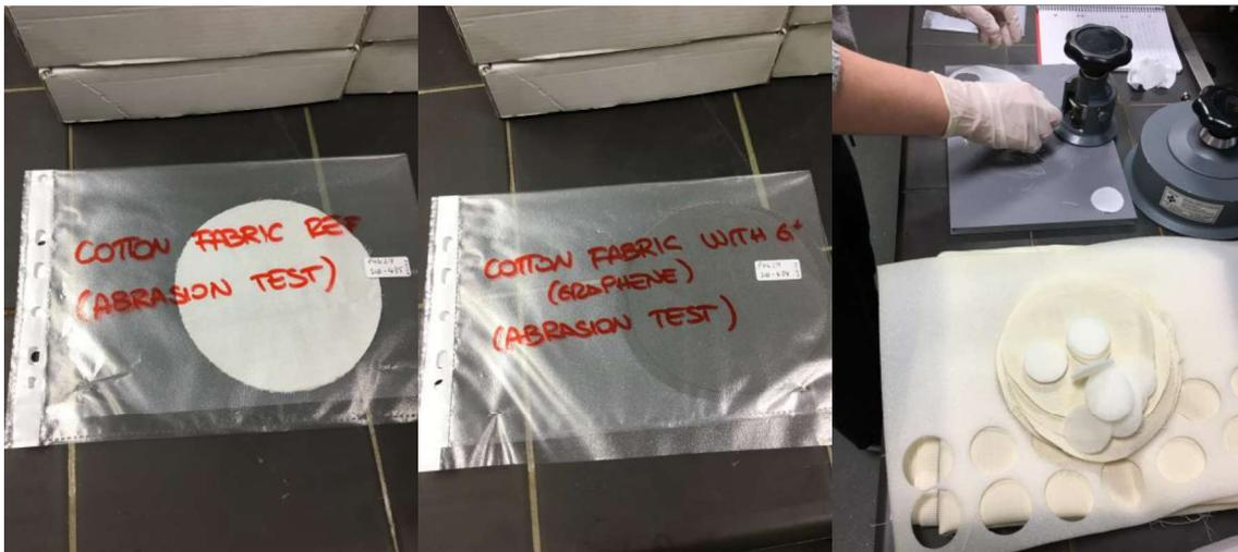
Figure 2.1 Cotton textile samples (left and middle) and polyetherurethane foam inserts cut to correct size (right)
