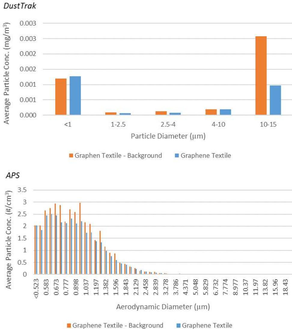
**Figure 3.4.** DustTrak and APS particle size distribution (PSD) graphs of the background period before the start of abrasion testing and for graphene-enhanced textile testing. DustTrak, size range <1 – 15  $\mu\text{m}$ . APS, size range 500 nm - 1  $\mu\text{m}$ .
