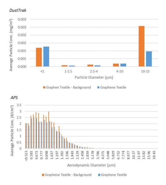
Figure 3.4. DustTrak and APS particle size distribution (PSD) graphs of the background period before the start of abrasion testing and for graphene-enhanced textile testing. DustTrak, size range  $<1-15 \mu m$ . APS, size range  $500 \text{ nm} - 1 \mu m$ .
