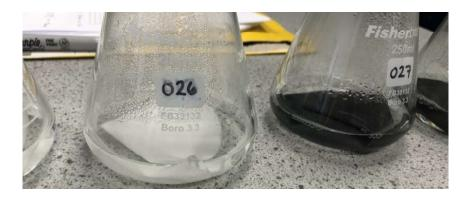
Figure 1 Cotton material samples were folded into the 250mL flasks (as provided at 10cm)
