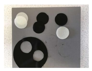
Figure 2.1 Textile samples and polyetherurethane foam inserts cut to correct size
