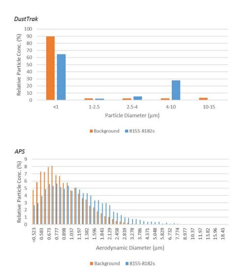
Figure 3.4. DustTrak and APS particle size distribution (PSD) graphs of the peak observed at the start of abrasion testing of graphene-enhanced textile (Figure 2.3, 8155 and 8182 s). DustTrak, size range <1 – 15  $\mu$ m. APS, size range 500 nm - 1  $\mu$ m.
