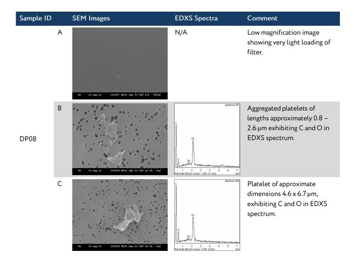
Very few particles were observed on the filters collected during abrasion sampling of the graphene-enhanced fabric. This is most likely due to the very short sampling time due to the reduced number of rubs to the fabric.
