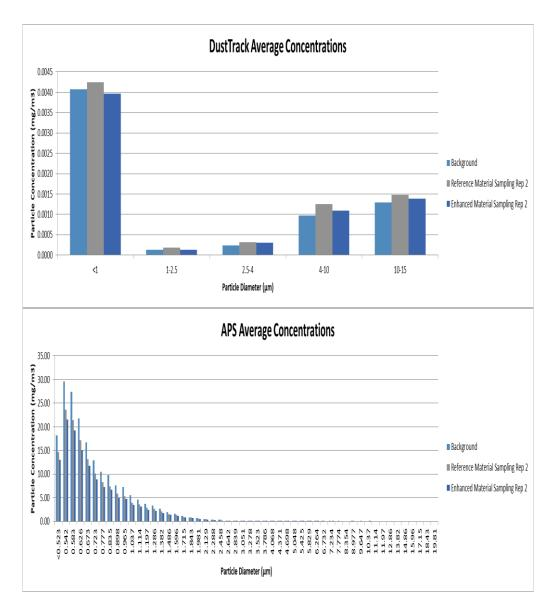
Figure 3.4. DustTrak and APS particle size distribution (PSD) graphs of the background period before the start of abrasion testing and for graphene-enhanced textile testing. DustTrak, size range <1 – 15 µm. APS, size range 500 nm - 1 µm.
