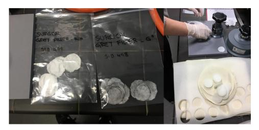
Figure 2.13 Layer TNT heat sealed textile samples (left) and polyetherurethane foam inserts cut to correct size (right)
