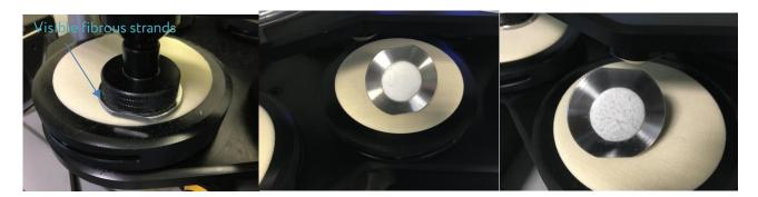
Figure 3.1 Image showing visible fibrous strands (left), wear to baseline fabric (middle) and abradant material (right).
