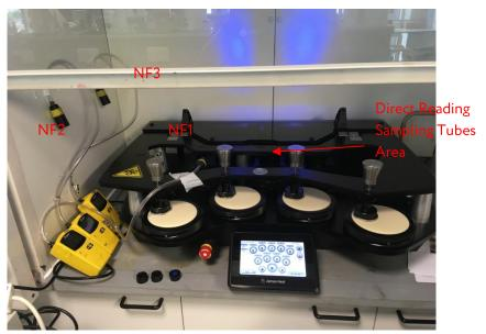
Figure 2.2 Image of Martindale instrument with static sampling and real-time sampling positions outlined
