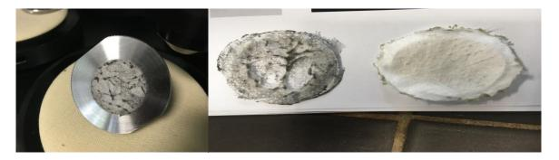
Figure 3.2 Image showing wear to graphene-enhanced fabric post-test (left) and post testing abradant materials (right).
