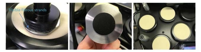
Figure 3.1 | mage showing visible fibrous strands (left), wear to baseline fabric (middle) and abradant material (right).
