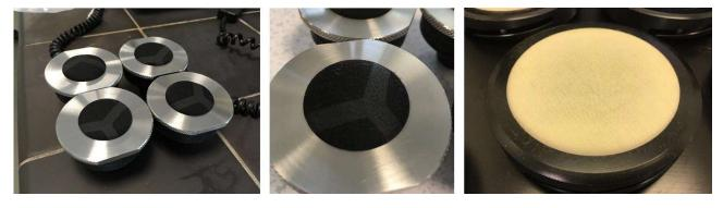
Figure 3.2 Image showing graphene-enhanced fabric before test (left), wear to graphene-enhanced fabric (middle) and abradant material (right).
