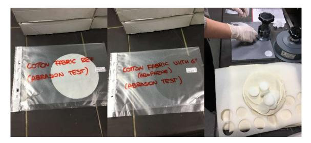
Figure 2.1 Cotton textile samples (left and middle) and polyetherurethane foam inserts cut to correct size (right)
