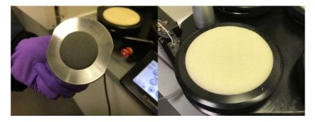
Figure 3.2 Image showing wear to graphene-enhanced fabric post-test (left) and abradant material (right).
