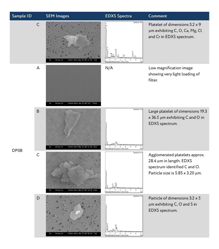
The particles on these filters exhibited a morphology and composition similar to what could be expected for graphene. However, material with a similar morphology was found on filters collected during testing of the reference cotton fabric, i.e. with no graphene coating (Table 3.4). It is therefore not possible to conclusively identify these platelets as graphene. The use of free graphene reference material for our own SEM analysis would
